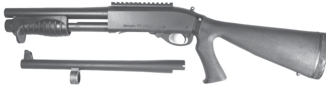
Figure 4.67 The Remington Modular Combat Shotgun. The MCS is based on Remington's 870 shotguns, with some upgrades to suit its purpose as a combat shotgun. (Image from author's collection.)
